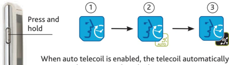
When auto telecoil is enabled, the telecoil automatically turns on when you use the telephone or enter a room loop environment. ③
